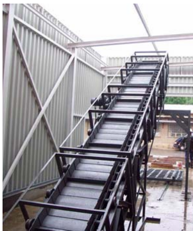
Metallic belt conveyor
