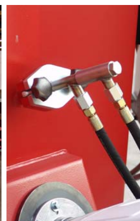
Injection system for liquid waste
